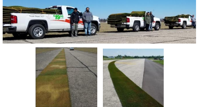
Figure 10. 450 m 2 surrogate grass on the test track.
