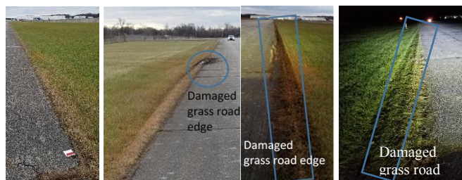
Figure 11. The real grass before and after run-over tests.
