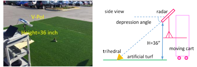
Figure 1. 77GHz radar horizontal polarization measurement setup.
