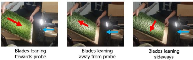
Figure 3. Leaning directions of artificial turf with respect to the measurement probe.
