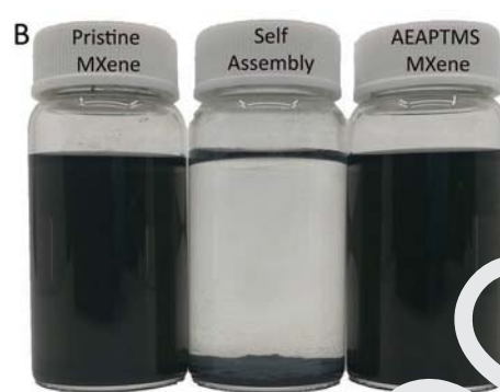
Figure 5. A) Surface charge of the pristine MXene and AEAPTMS- \text{Ti}_3\text{C}_2\text{T}_x versus pH, and B) self-assembled film obtained from mixing the positively charged functionalized MXene and the negatively charged pristine MXene.
