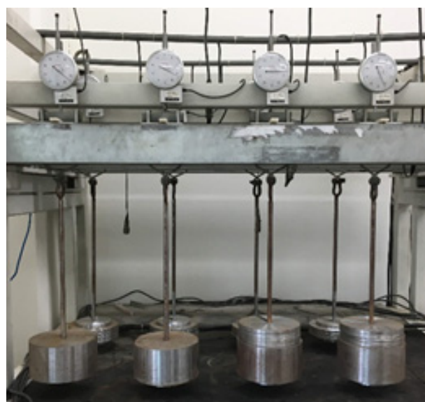
Fig. 4. Creep test loading.
