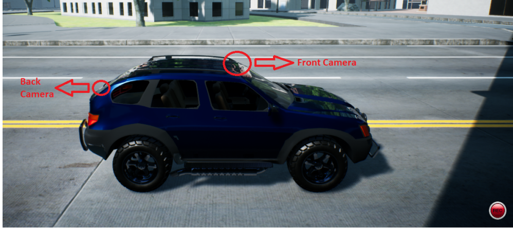
Figure 4.1. The locations of front and back cameras on the vehicle.
