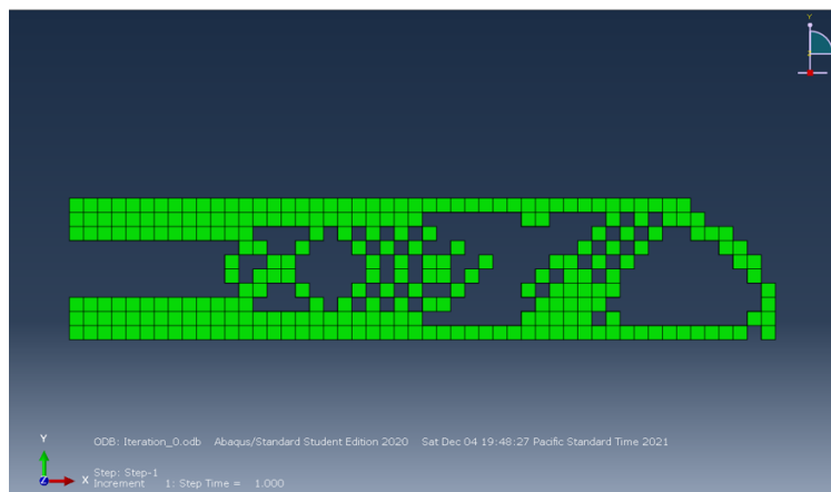
Figure 6.8. HCA 2D Element Optimized Structure (Iteration 200 )
