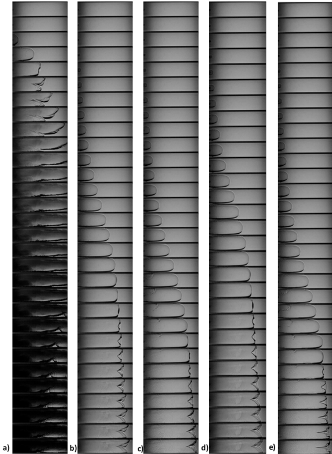
Figure 3.2. Schlieren filmstrips for five 50%-50% methane-hydrogen ( \Phi=1 ) test cases: a) Trial 186: \tau_{\text{mix}}=0\text{s} , no pump; b) Trial 190: \tau_{\text{mix}}=10\text{s} , no pump; c) Trial 210: \tau_{\text{mix}}=10\text{s} , pump; d) Trial 194: \tau_{\text{mix}}=30\text{s} , no pump; e) Trial 214: \tau_{\text{mix}}=30\text{s} , pump.
