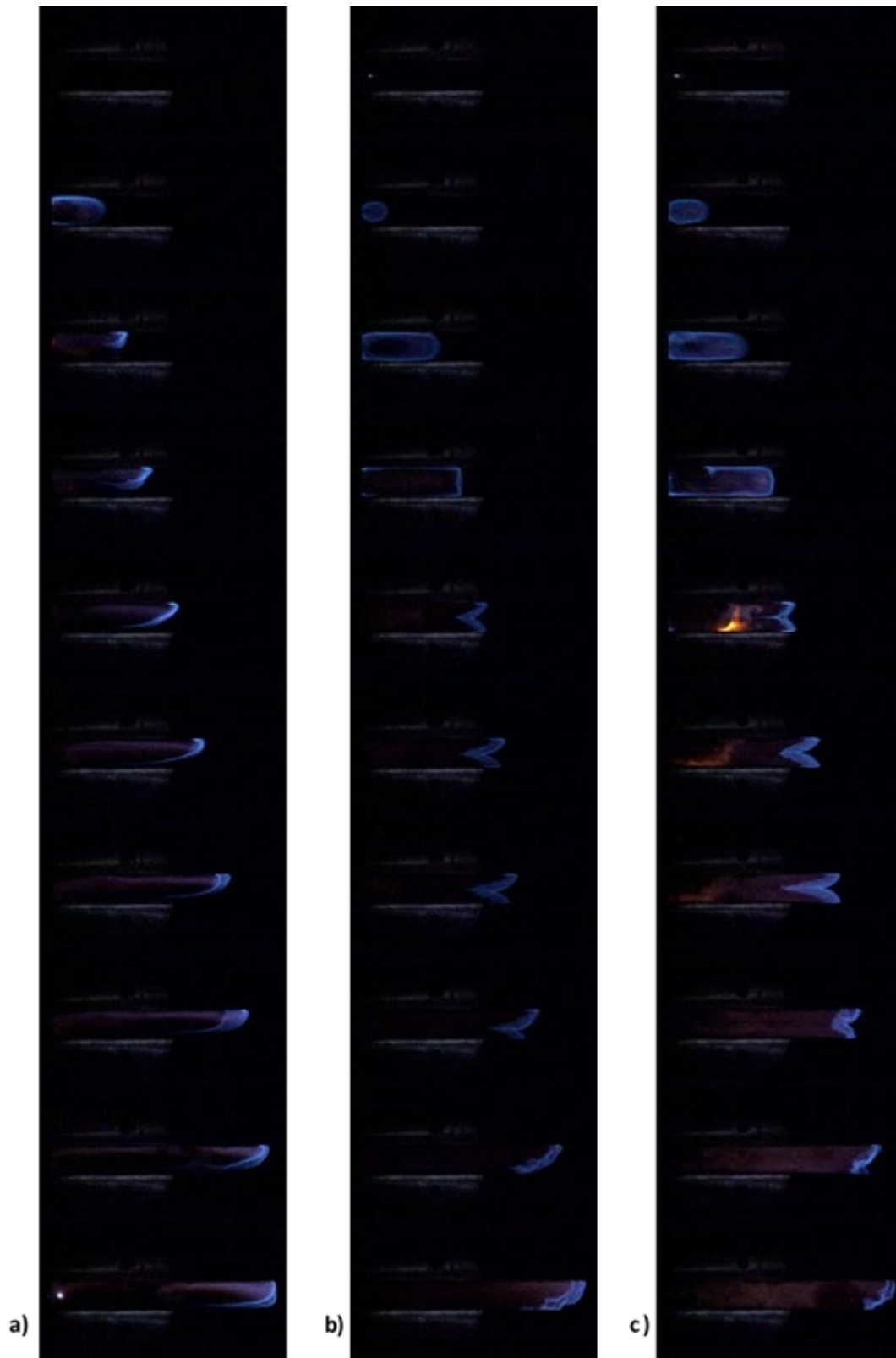
Figure 3.7. Flame luminosity filmstrips for 3 methane-hydrogen ( \Phi=1 ) test cases: a) Trial 186: \tau_{\text{mix}}=0\text{s} , no pump; b) Trial 194: \tau_{\text{mix}}=30\text{s} , no pump; c) Trial 214: \tau_{\text{mix}}=30\text{s} , pump.
