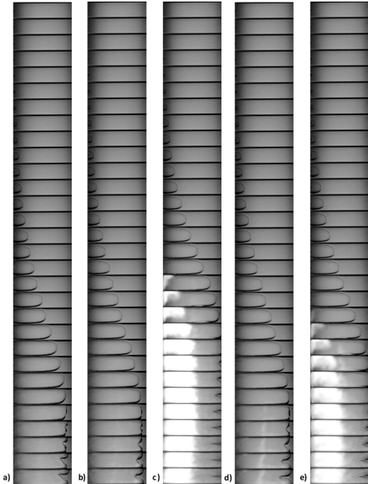
Figure 3.3. Schlieren filmstrips for five hydrogen ( \Phi=1 ) test cases: a) Trial 235: \tau_{\text{mix}}=0\text{s} , no pump; b) Trial 239: \tau_{\text{mix}}=10\text{s} , no pump; c) Trial 260: \tau_{\text{mix}}=10\text{s} , pump; d) Trial 241: \tau_{\text{mix}}=30\text{s} , no pump; e) Trial 263: \tau_{\text{mix}}=30\text{s} , pump.
