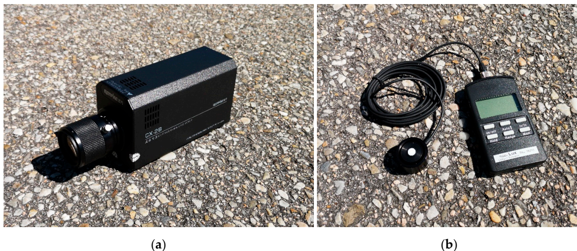
Figure 4. Measurement equipment used to collect luminance and illuminance data: (a) CX-2B imaging luminance meter; (b) Mobilux luxmeter.
