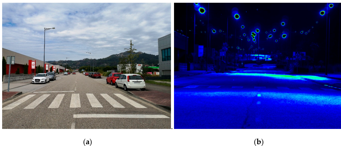
Figure 7. Road lighting installation considered to verify the methodology: (a) picture of the real scenario; and (b) luminance image photographed with the luminance meter.
