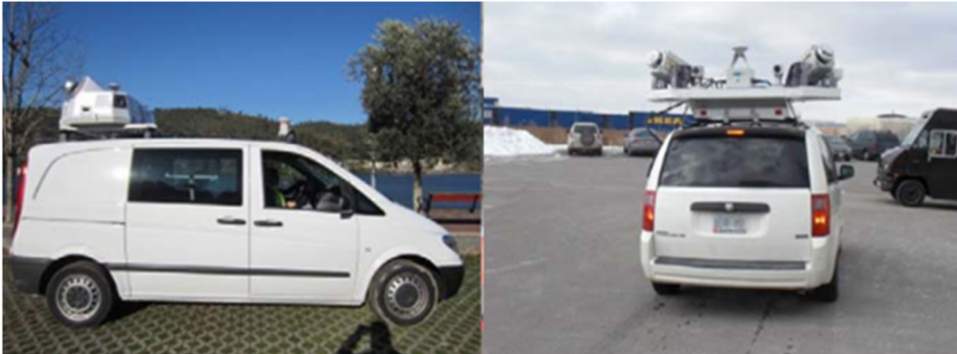
Figure 2. Mobile LiDAR System used for the survey.
