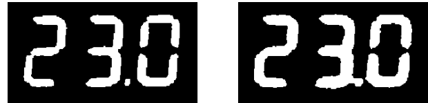
Fig. 6. Left: Peak detection method. Right: iterative Otsu method.
