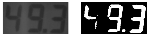
Fig. 7. Left: Image with illumination gradient. Right: binarization with a single threshold.
