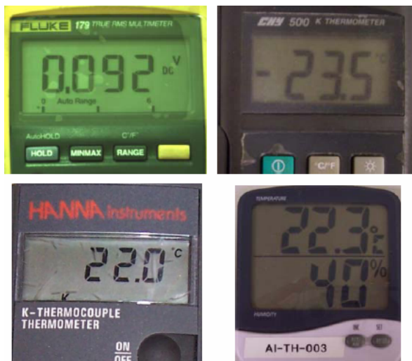
Fig. 1. Examples of different instruments, some of them are showing display defects (bubbles in the first one, stripes in the third one).
