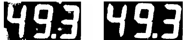
Fig. 8. Images binarized with interpolated thresholds. Left: 8x8 sub-images. Right: 4x3 sub-images.
