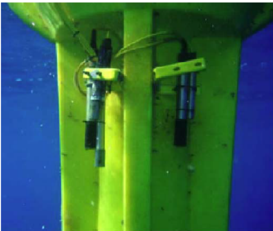
Fig. 3.- Sensor arrangement: classical buoy (left), Hidroboya (right).
