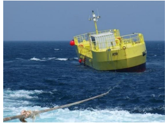
FIGURE 33 Roll and yaw of the Atir platform during tests with only one turbine running
