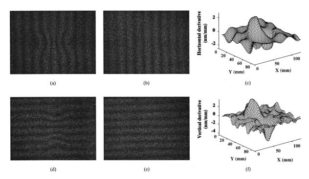
**Fig. 3** Transient bending waves in a metal plate 25  $\mu$ s after mechanical excitation: (a) to (c), horizontal shear; (d) to (f), vertical shear; (b), (e), carrier fringes; (a),(d), corresponding double-pulsed-subtraction TV shearography fringe patterns, deformation plus carrier; (c), (f) three-dimensional plots of the spatial derivatives of the out-of-plane displacement.
