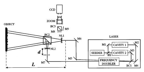
**Fig. 2** Schematic experimental setup used to generate carrier fringes in double-pulsed-subtraction TV shearography: BS, beamsplitter; BC1 to BC3, beam combiners; M1 to M9, mirrors; NL1 and NL2, negative lenses (their foci are shifted by a distance *d*).
