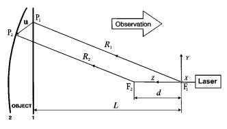
Fig. 1 Geometry of the optical-path separation approach.
