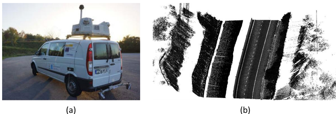
Figure 1. Case study data. (a) Optech LYNX Mobile Mapper. (b) Raw point cloud section.
