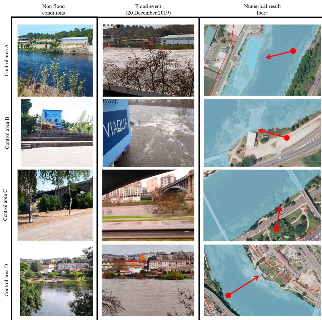
Figure 6. Results of flood extent for each control area. First column depicts non-flood conditions ( Q = 265 \text{ m}^3 \text{ s}^{-1} that corresponds to 66th percentile) at the control areas. The second column shows the images (photographs taken by one of the authors) of the flood event (20 December 2019, 16:00 to 16:30) and the third column shows the numerical results obtained with Iber+. Red arrows in the third column represent the direction of the photograph taken during the flood event.
