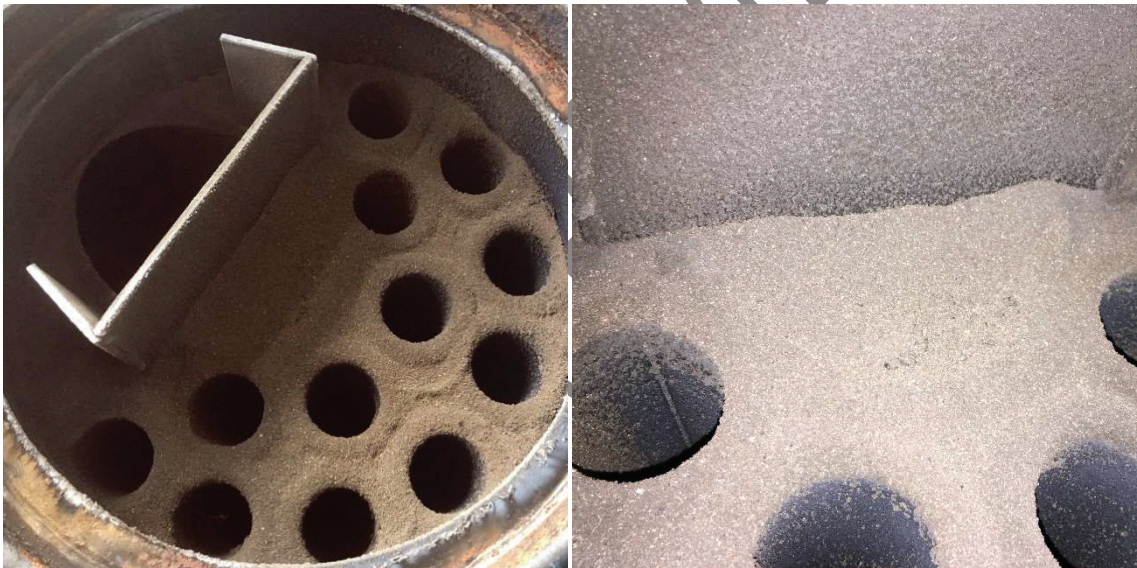
Figure 11. Experimental run. Fouling on top surface due to gravitational settling.
