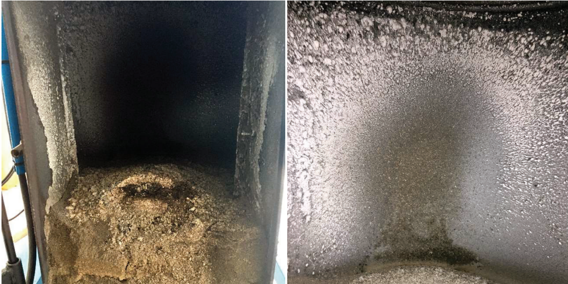
Figure 10. Experimental run. Left, fouling on front access door. Right, annular shape of the fouling on the combustion chamber surface.
