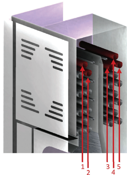
Fig. 5. Location of the 5 tubes where the sampling probes are placed.
