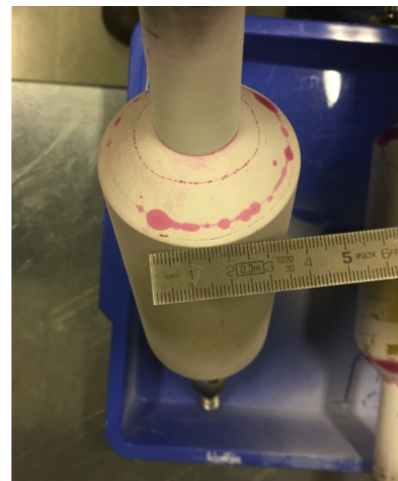
Figure 10: Observation of defective regions on IB30kV2, revealed by the application of liquid penetrant.
