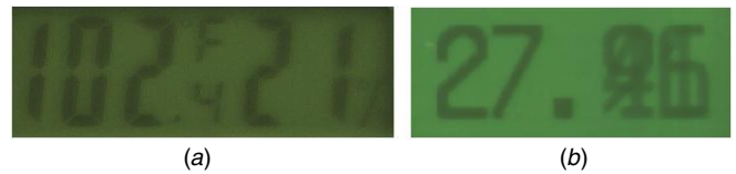
Figure 15. Problematic displays: (a) special display; note F above the decimals and (b) display in transition.
