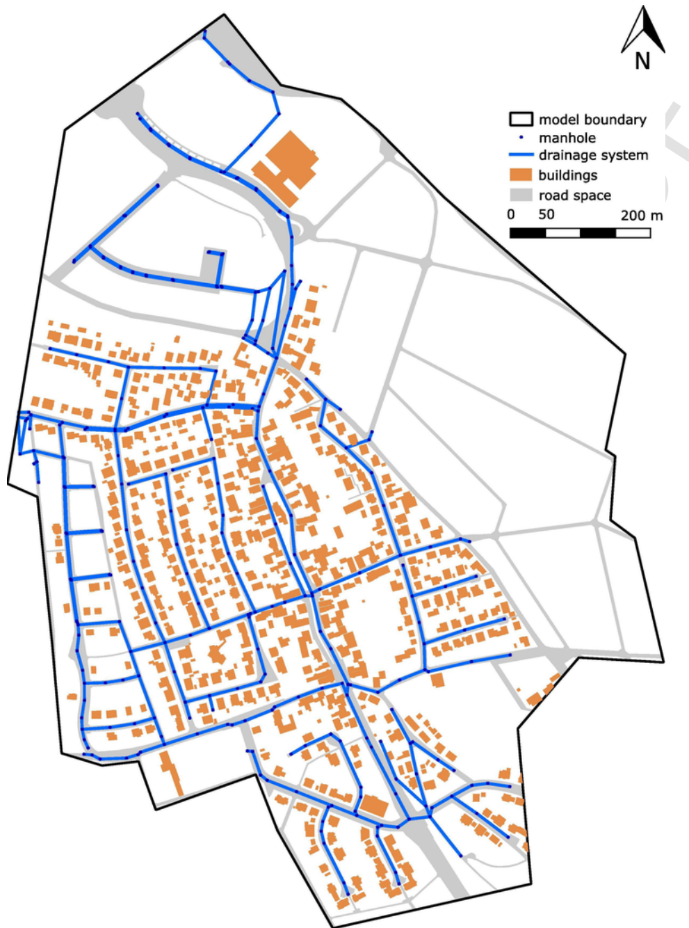
Fig. 4. Schematic representation of test area 2, including the elements of the drainage system, road space and buildings.
