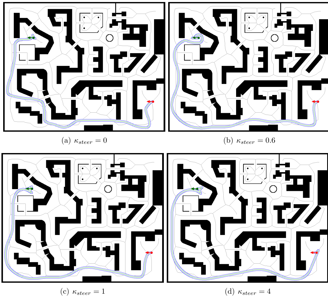
Figure 7.11: Produced global paths with different settings of \kappa_{steer}
