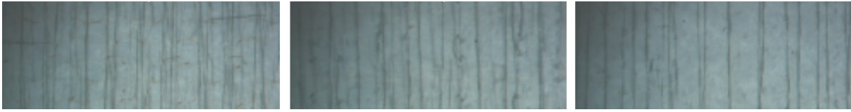
Figure 2.11: Strain rate dependent crack densities in biaxial weft-knitted fabric, increasing strain rate from left to right, Hufenbach (2007)
