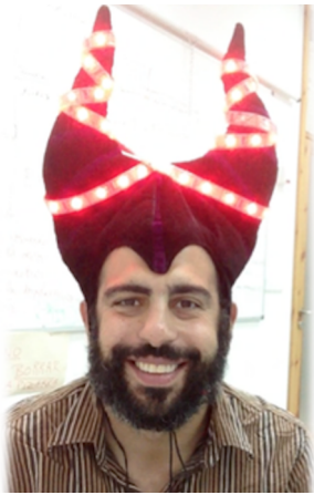
Figure 1: The StimuHat interface consists of a hat augmented with LED lights and biosignal sensors.
