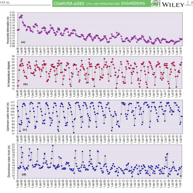
FIGURE 2 Time series monitoring data: (a) horizontal deformation (HD; m) at the PV6 station and (b) air temperature (°)
