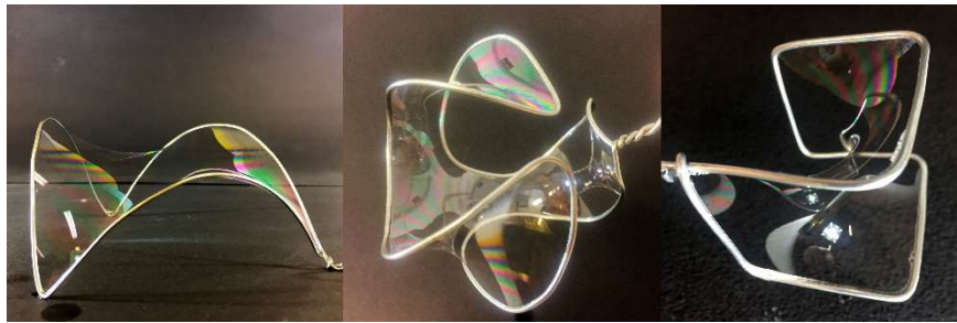
Fig. 3 Minimal surface physical models obtained using a bent wire without self-intersections, which acts as a rigid edge. Generation of the Scherk surface on the right. Images: authors
