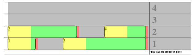
Fig. 3. Example of Always off policy. On (green), Shutting Down (red), Off (grey), Booting (yellow). (For interpretation of references to colors in this figure legend, the reader is referred to the web version of this article.)
