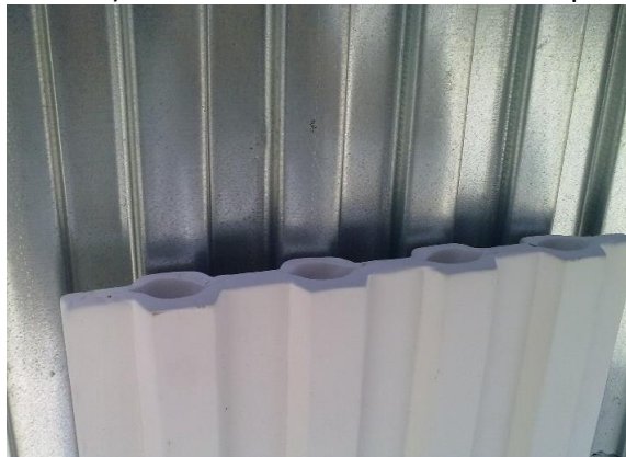
Figure 5 Porous ceramic cladding tile designed for SOLARKIT's ventilation towers
