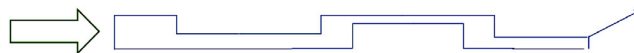
Figure 4. Cross section through a strip of muscovite crystal that shows no continuous layers between the irradiated end and the exit terminal. The arrow to the left represented the flow of alpha particles and the small arrow to the right the connection to the metering instruments. The c axis of the crystal is vertical. The result does not depend on the orientation of the other axes as it has been shown that quodons can scatter into any of the chain directions and then move by percolation. Of course, it can be expected that the charge moves fastest if a chain is parallel to the line of the cable.
