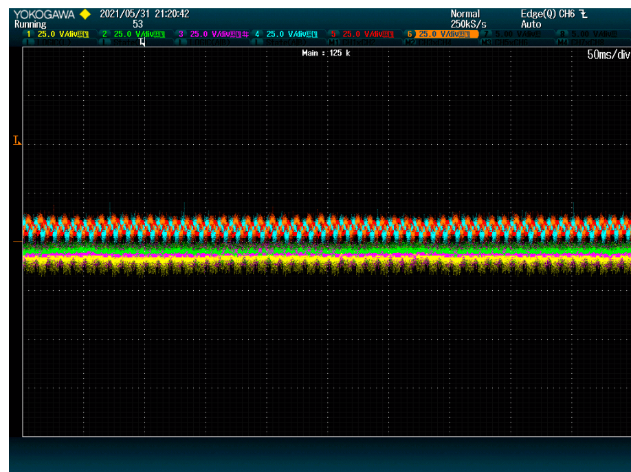
Figure 11. Modules DC-Link voltage when reducing ripple. The plot shows voltage (25 V/div) vs. time (50 ms/div).
