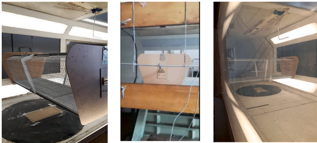
Fig. 14. The model installed in the wind tunnel.
