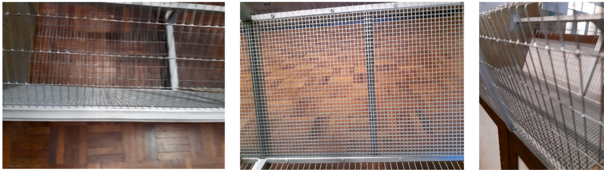
Fig. 13. The model's deck beam, floor mesh and guard mesh.
