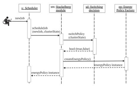
Fig. 4. Sequence diagram of the interactions between modules of the Stackelberg Game workflow
