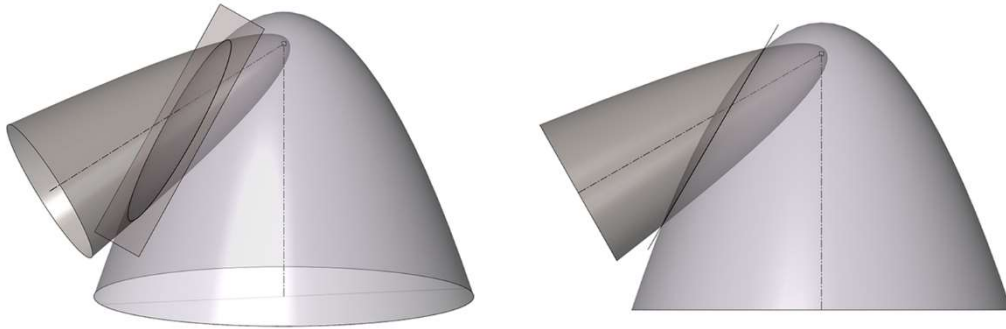
Fig. 14. Paraboloid-Paraboloid intersection. The intersection between two paraboloids sharing the position of a focus at the same "real" point is a planar curve, and, in general, an ellipse. This supports the initial hypothesis. Source: Authors' own
