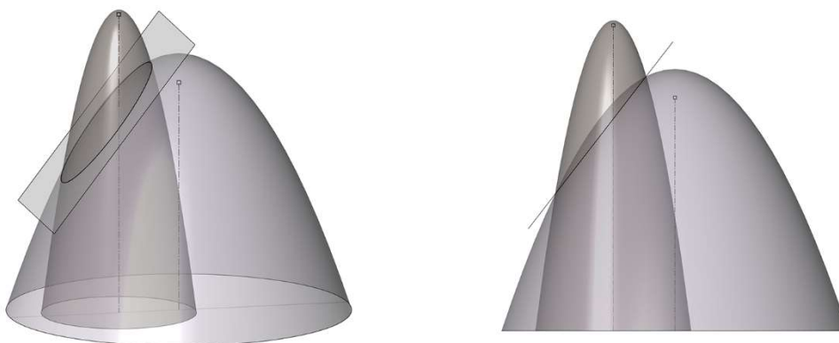
Fig. 13. Paraboloid-Paraboloid intersection. The intersection between two paraboloids sharing the position of a focus at the same "ideal" point (the two surfaces have parallel axes that meet at a point of infinity) is a planar curve, and, in general, an ellipse, which would degenerate into a parabola if both paraboloids had the same scale. This supports the initial hypothesis. Source: Authors' own
