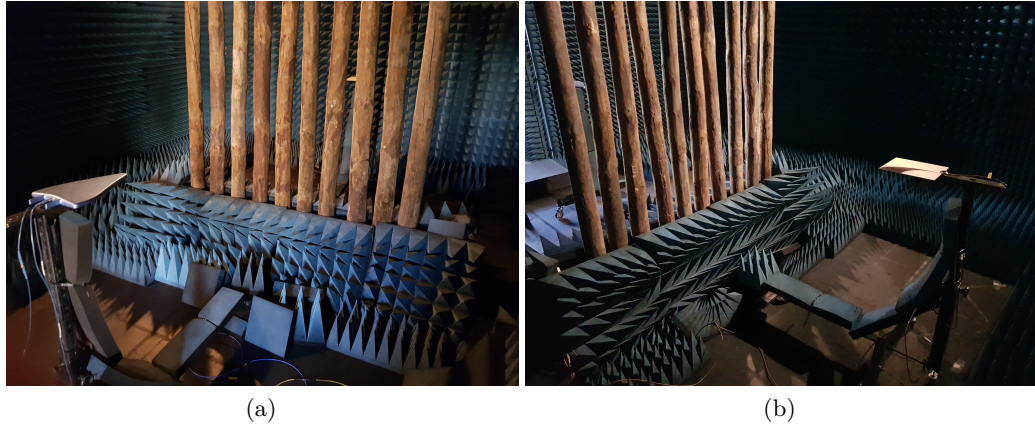
Figure 43: The assembled barrier and equipment from the perspective of TX (a) and RX (b).
