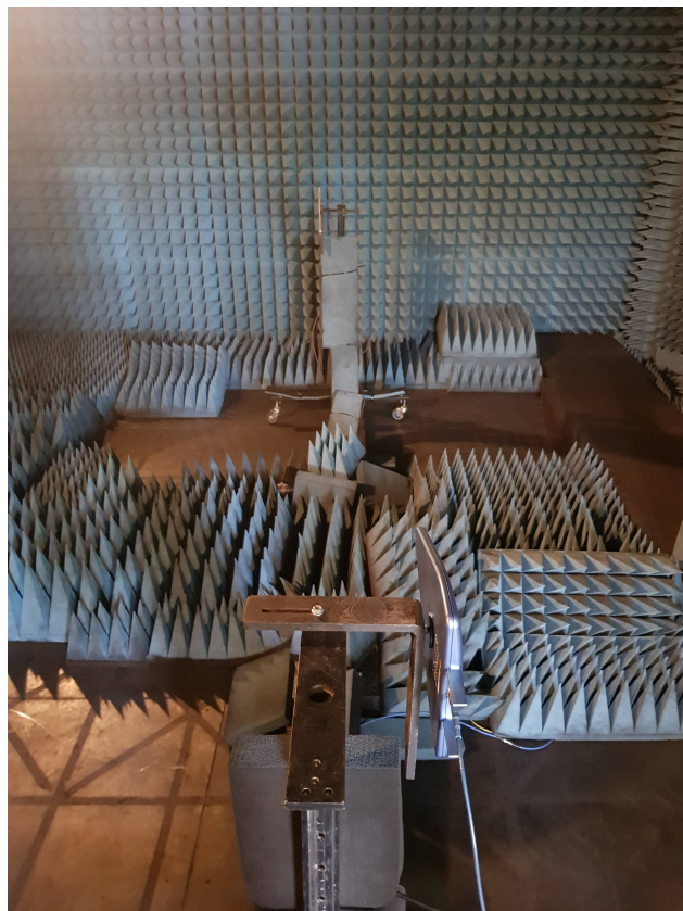
Figure 44: Setup for free space measurements.
