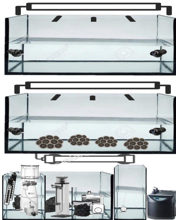
Figure 5- Illustration of the aquarium system composed of two aquariums and with the filtration system located in the sump.
