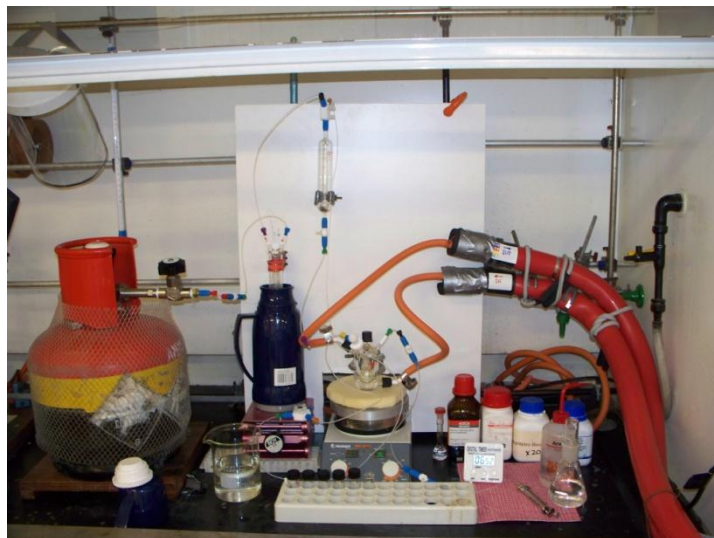
Figure 9 Diagram of the set-up of pressure equipment for the studies in liquid ammonia. B, C and D are fixed into a 60 × 40 cm wooden board by clamps. B and C are placed inside a wooden protection box with a Perspex sheet as front window and a protection sheet is placed in front of D when A is charged with liquid ammonia. The maximum working temperature allowed for the system is 45 °C (18 bar).
