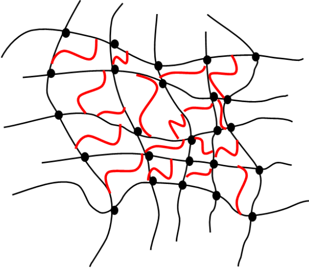
Figure 3: Schema of strongly crosslinked polymer chains with added oligomers without functional groups (red lines).
