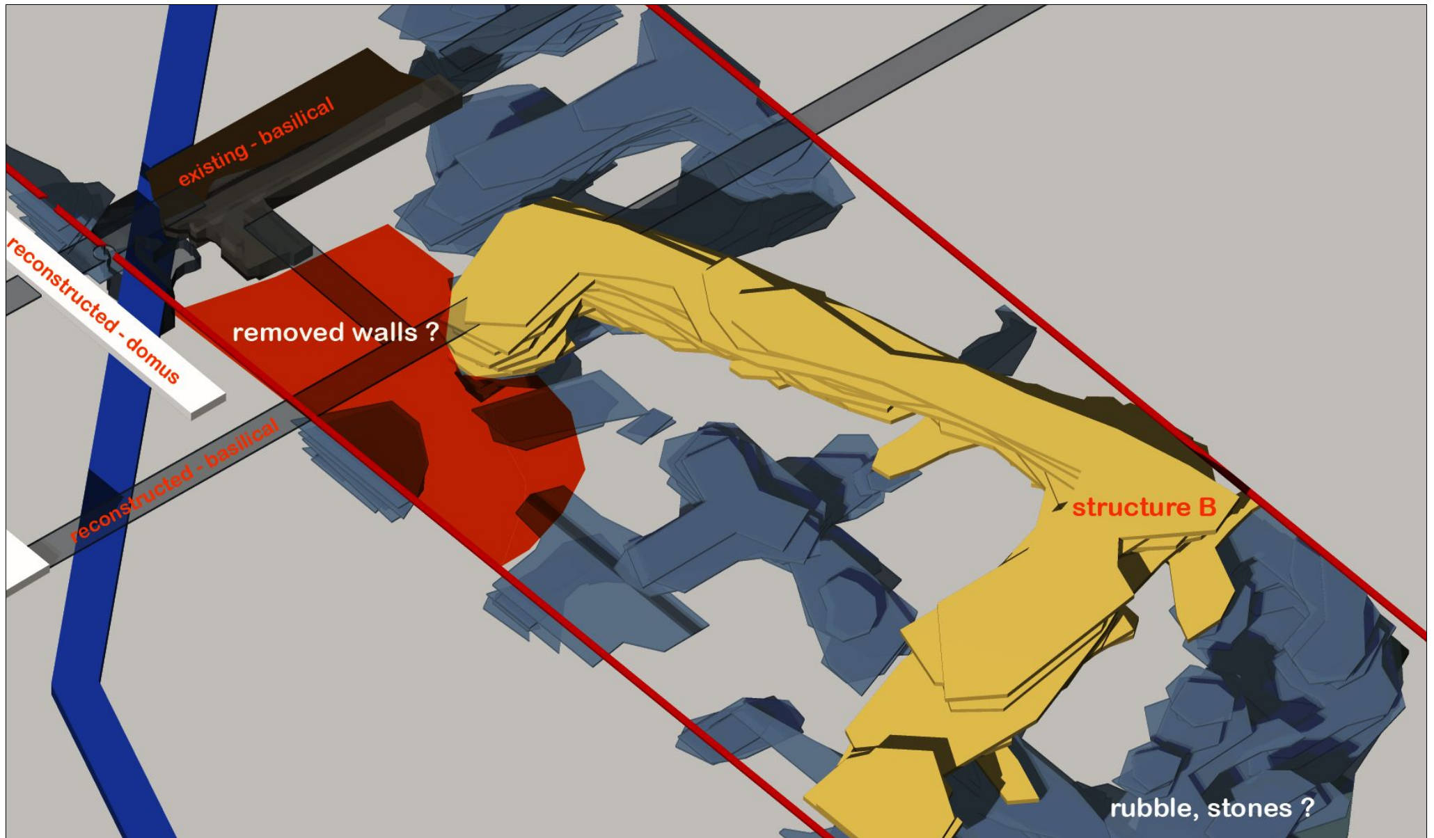
Fig. 6. Close view of GPR test-area 4, showing the connection between excavated and GPR surveyed structures.
