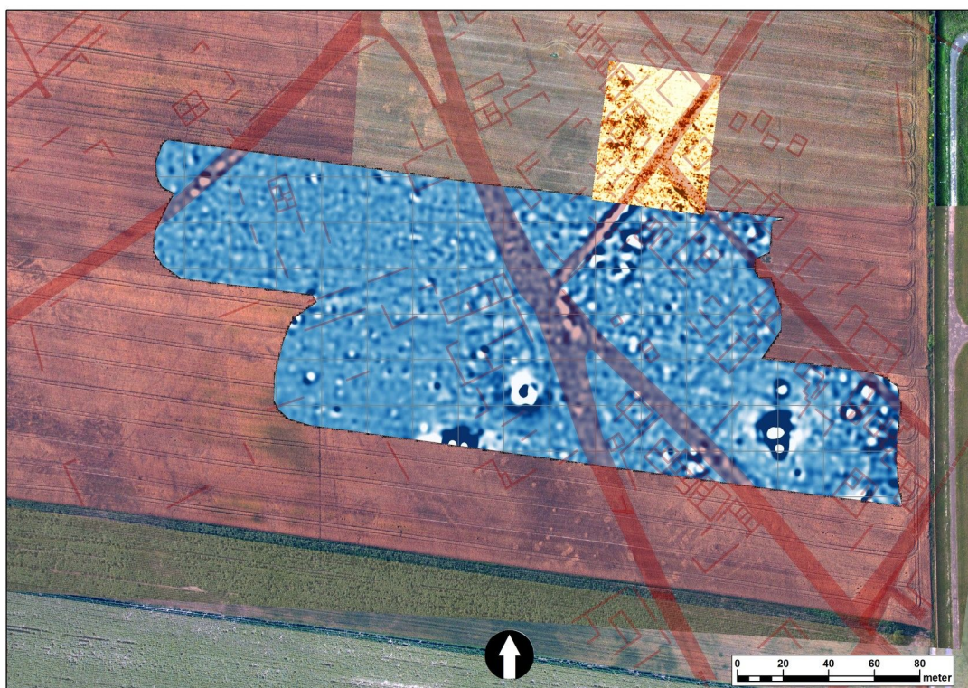
Fig. 3. Remote sensing topographical work at the northern part of the canabae. Magnetometer measurements (blue), GPR survey and aerial photography (brown).
