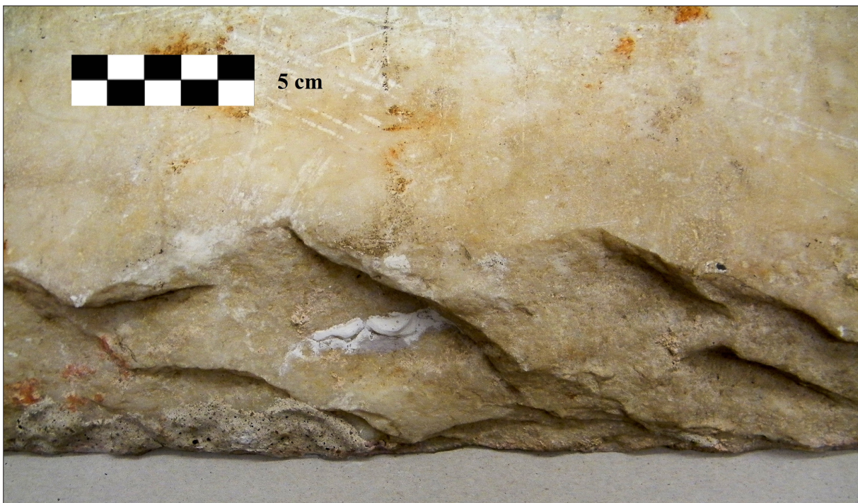
Fig. 5. Hammer marks on the lateral side of a marble element (54.437.125.).
