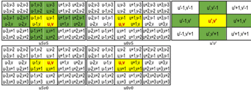
Fig. 4. Example of patch feature descriptors with R = 1 . Patches in Pixel Coordinate (u, v) ; u5v5 , u0v5 , u5v0 , u0v0 are reference patch feature descriptors of size 3 \times 3 pixel, which are generated from 6 \times 6 – pixel patches by average pooling from the reference image; and u'v' is target patch feature descriptor of size 3 \times 3 pixel.
