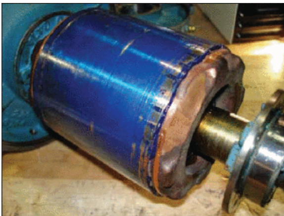
Figure 5 The die-cast copper rotor for an induction motor.
