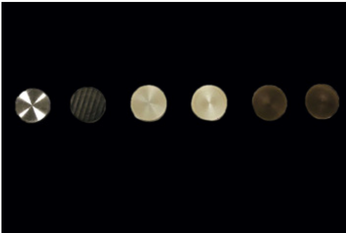
Figure 1. Experimental groups, left to right: Ti (machined Ti), TiL (Ti laser-treated), P (machined PEEK), PP (PEEK plasma-sprayed), PL (PEEK laser-treated), PLP (PEEK laser-treated and plasma-sprayed). PEEK, polyetheretherketone.
