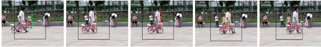
Figure 8.4: Illustration of the three states of the tracker. Black, green, yellow and red squares show the search areas, target found, partially lost and fully lost states.
