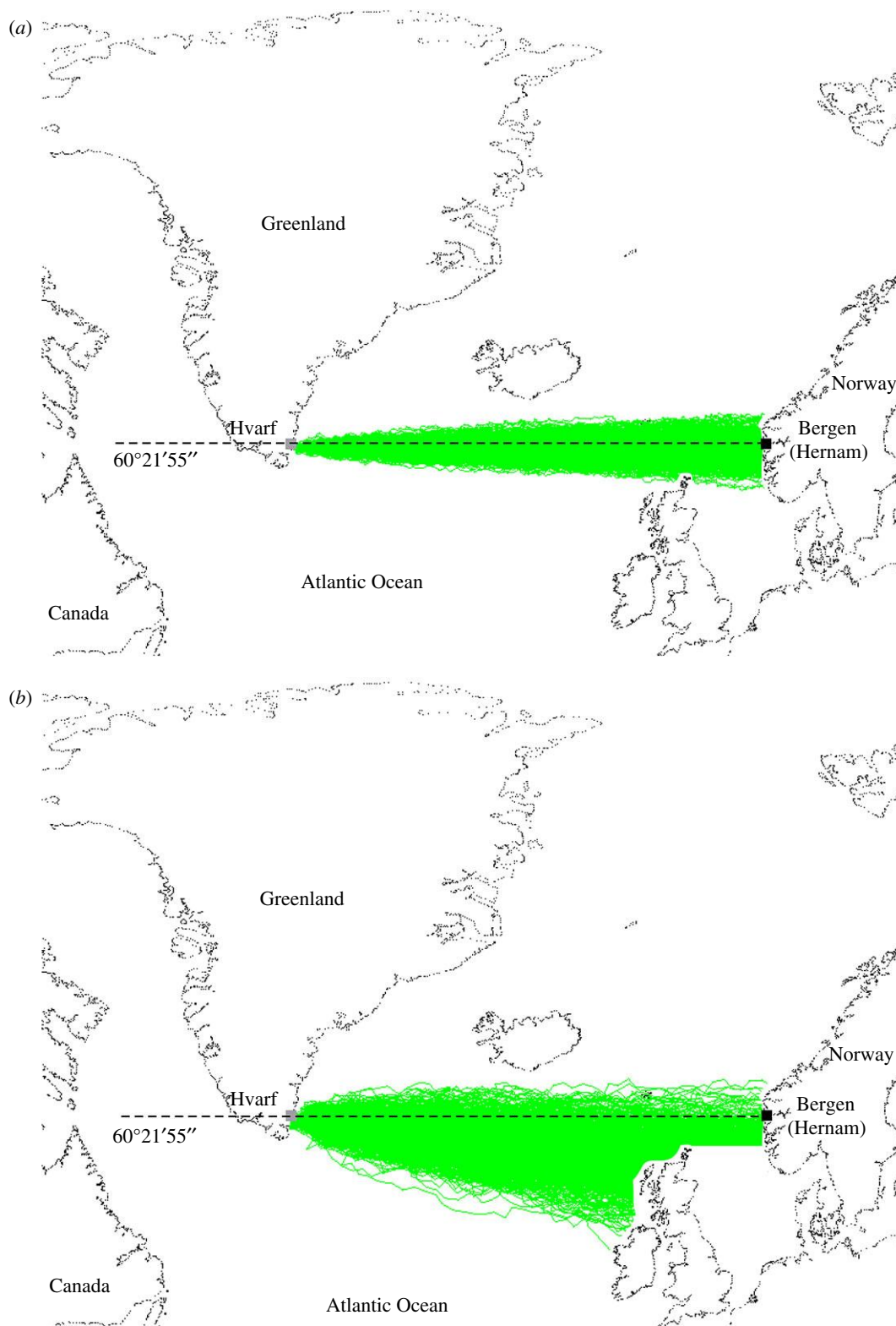
Figure 3. Simulated Viking sailing routes from Greenland to Norway. Simulated (successful: green) routes of 1000 Viking voyages from Hvarf (Greenland) to Norway at spring equinox, if a calcite sunstone crystal is used to analyse sky polarization with a navigation periodicity (a) \Delta t = 1 h, and (b) \Delta t = 6 h.
