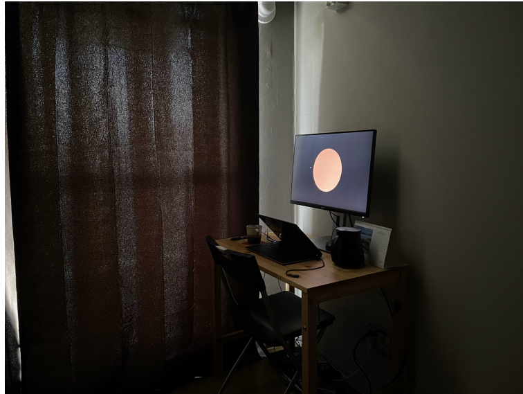
Figure 3.2: Data collection setup. This photo was taken during the day. The experiment was carried out at night, when the room was darker. It is interesting to note the monitor’s backlight bleed, which is a factor likely to affect the experiment.
