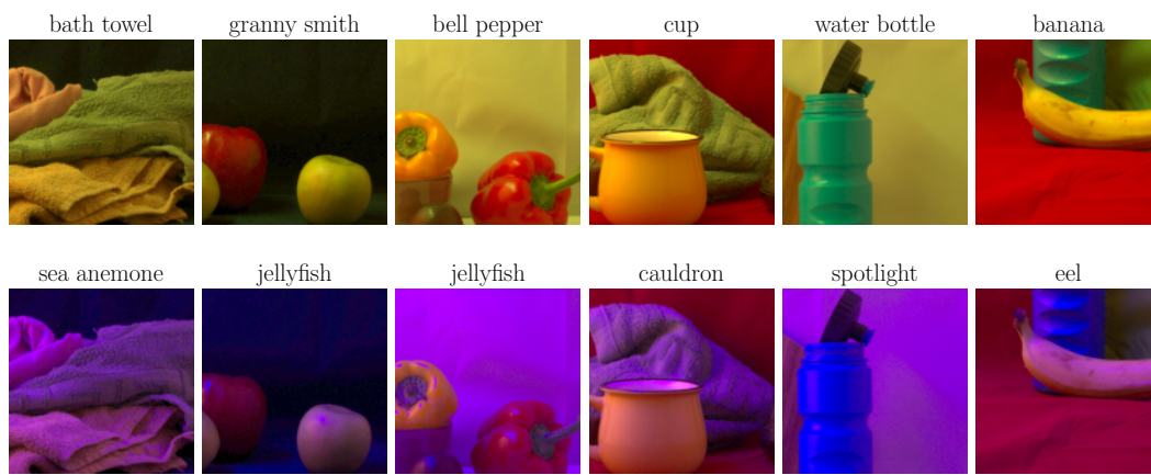
Figure 2.7: Scene-crop pairs where classification is correct in the best illumination and incorrect in the worst illumination. Only 1 of the 5 crop is shown per scene. Some, but not all, of the other 4 crops experienced the same classification results.
