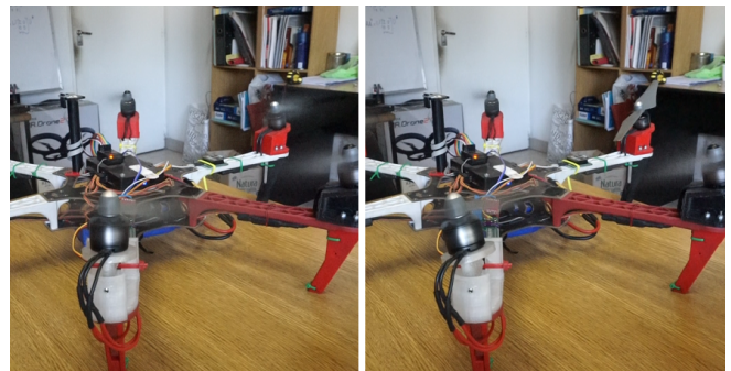
Figure 3: Servomotor in rotor 1 in the case without failure (left) and in the case of a failure in rotor 3 (right).
