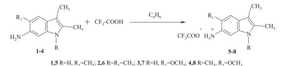
Scheme 1. Scheme for the synthesis of 1*H*-indol-6-ylammonium trifluoroacetates 5–8 from 1*H*-indol-6-ylamines 1–4 and trifluoroacetic acid.
