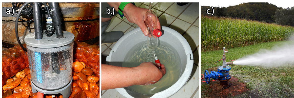
Fig. 2 Example of sampling sites: a Kraljevi vrelec, b V-3/66-70 water and gas after the separator and c gas lift at K-2/75. All have lots of free gas and show iron scaling (notice orange precipitates ( a , c ) and brownish colour in the bucket ( b ))
