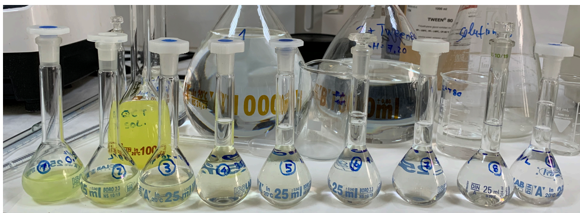
Figure 4 – Preparation of the nine standard solutions.
