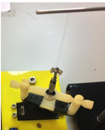
Fig. 2.14. Turning four separated wires into one single tetrode.
