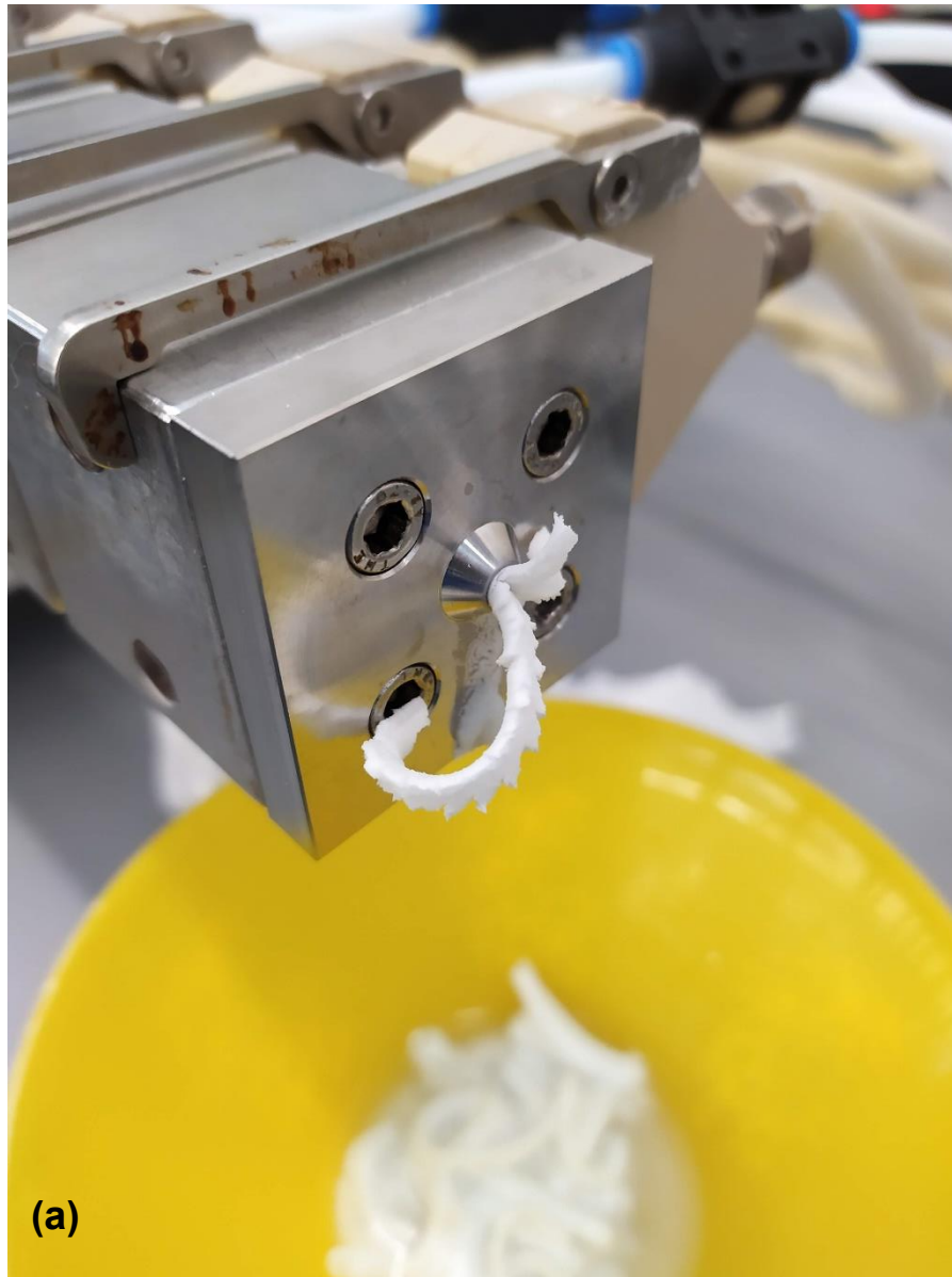
Appendix 1: Common defects observed in extrudates. (a) AM1 extrudate strand exiting the end-plate die. "Sharkskin effect" visible. (b) AM2 extrudate strand exiting the end-plate die. "Sharkskin effect" visible. (c) DCW 200 rpm extrudate strand exiting the end-plate die. Bubble-like areas visible.
