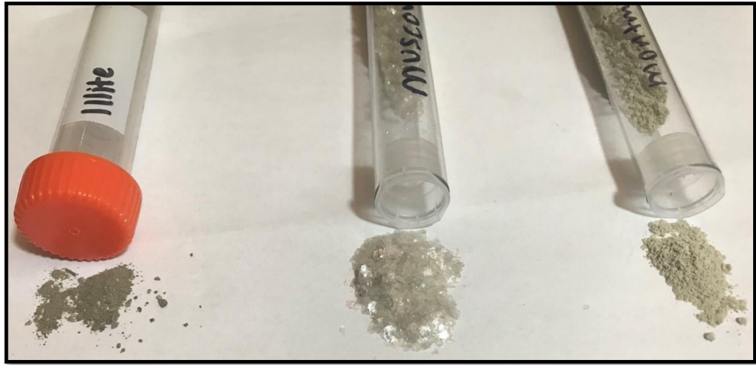
Figure 1.10. Phyllosilicate minerals investigated in this study: illite, muscovite, and montmorillonite.
